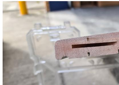
**3** Apply exterior grade wood glue into both halves of the biscuit rebate and to one face of the end grain
