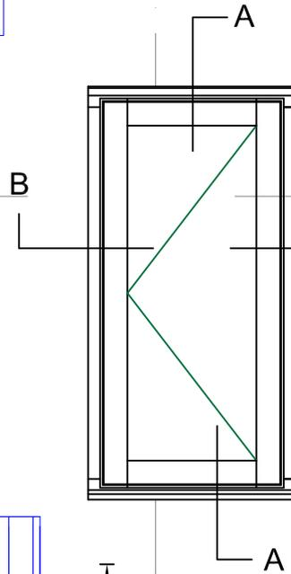
Typical sections showing acoustic glass - 8.8Aku/16ar/6T (**42 dB**)
