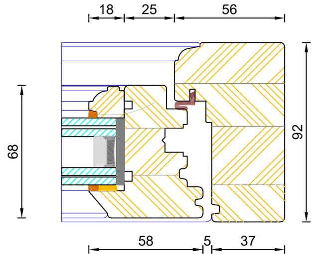
Typical sections showing acoustic glass - 9.5/16Ar/8.8Aku T CG A 1.0 (45dB)
