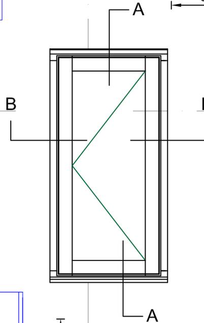
Typical sections showing acoustic glass - 8.8Aku/12ar/4T (39 dB)
