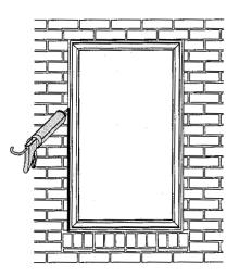
A minimal expansion gap filling foam should be used post fixing to seal the frame into the fabric of the building creating and air and watertight seal.
