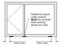
Support packers should be located at all fixing points. If additional packers are required to raise the position of the frame in the aperture or to compensate for the base of an aperture that is not level, all mullions must be supported.
